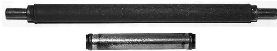
Fig. 5. Original (above) and surface coated (below) test tubes after 2000 h exposure to LBE flowing with 1–1.2 m/s at 550 °C; the original one shows a dark layer, the surface coated one is still shiny.
